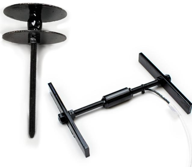
ASPHALT STRAIN TRANSDUCERS (AST/VAST) MEASURE AXIAL STRAIN IN FLEXIBLE PAVEMENT UNDER HIGH FREQUENCY (DYNAMIC) CONDITIONS. THESE LOW MODULUS, RUGGEDIZED SENSORS ARE BUILT TO WITHSTAND THE HIGH TEMPERATURE AND VIBRATORY ROLLED COMPACTION REQUIRED FOR ASPHALT PLACEMENT.
