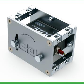
THE T500 TILTMETER IS AN **ELECTROLYTIC FLUID-BASED TILT SENSOR THAT CAN BE USED FOR PRECISION ROTATION** MEASUREMENTS, GENERALLY OVER A SHORT PERIOD OF TIME. THESE UNITS CONNECT DIRECTLY TO OUR STRUCTURAL TESTING SYSTEM, STRUCTURAL MONITORING SYSTEMS, AND ARE ALSO COMPATIBLE WITH MOST GENERIC DATA ACQUISITION SYSTEMS. THE RUGGED ALUMINUM HOUSINGS PROVIDE BOTH EASY MOUNTING AND MECHANICAL ZERO-ADJUSTMENT CAPABILITY.
