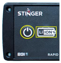
Figure 8: Power Button on the left and Battery Indicator Button on the right
