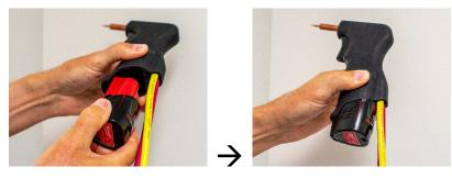
Figure 2: Lithium-ion Battery Installation
