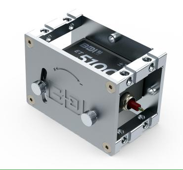
THE T500 TILTMETER IS AN **ELECTROLYTIC FLUID-BASED TILT SENSOR THAT CAN BE USED FOR PRECISION ROTATION** MEASUREMENTS, GENERALLY OVER A SHORT PERIOD OF TIME. THESE **UNITS CONNECT DIRECTLY TO OUR** STRUCTURAL TESTING SYSTEM, STRUCTURAL MONITORING SYSTEMS, AND ARE ALSO COMPATIBLE WITH MOST GENERIC DATA ACQUISITION SYSTEMS. THE RUGGED ALUMINUM **HOUSINGS PROVIDE BOTH EASY** MOUNTING AND MECHANICAL ZERO-ADJUSTMENT CAPABILITY.
