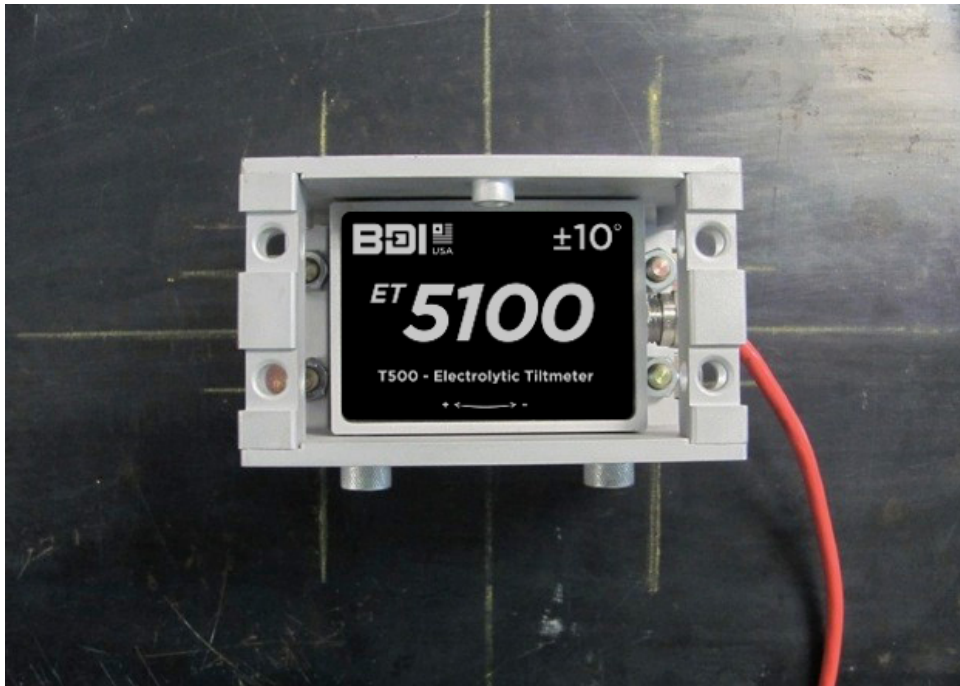
Figure 12: Tiltmeter Installed on Structural Member
