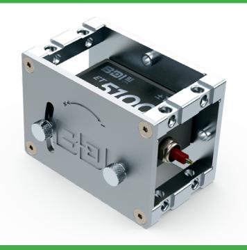
THE T600 TILTMETER IS A SINGLE OR DUAL-AXIS MEMS-BASED SENSOR THAT CAN BE USED IN BOTH SHORT-TERM TESTING AND LONG-TERM MONITORING APPLICATIONS. WITH OVER-DAMPING IN THE SENSING **ELEMENT, THEY ARE LESS** SENSITIVE TO VIBRATION MAKING THEM MORE SUITABLE FOR HIGHER FREQUENCY RESPONSES. THE **RUGGED ANODIZED ALUMINUM** HOUSING PROTECTS AGAINST THE HARSHEST ENVIRONMENTS WHILE PROVIDING SIMPLE MOUNTING **OPTIONS AND MECHANICAL** OFFSET ADJUSTMENT.
