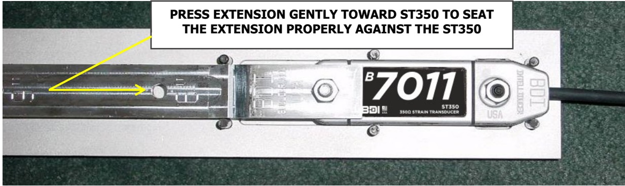
Figure 17: Aligning ST350 and Extension in the Jig
