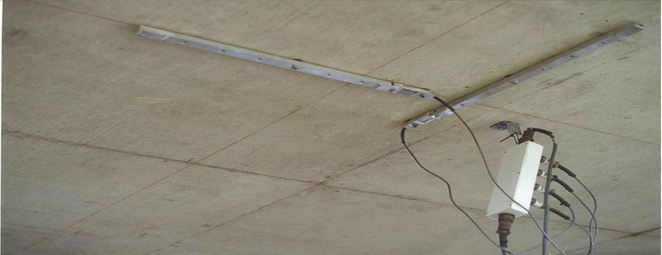
Figure 20: ST350 With Extensions Attached to an R/C Structure
