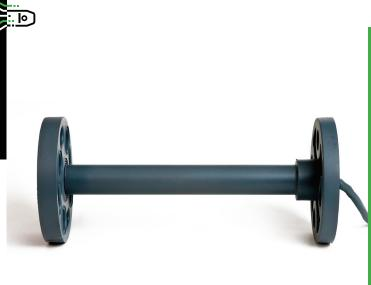
SOIL COMPRESSION SENSORS (SCS) MEASURE HORIZONTAL OR VERTICAL DISPLACEMENTS IN SOILS OR SUBGRADE MATERIAL. SCS'S ARE RUGGEDIZED TO WITHSTAND THE HARSH ENVIRONMENT IN SOILS AND CONSTRUCTION FILL MATERIAL DURING PLACEMENT AND COMPACTION. THESE GAGES ARE MOISTURE PROOF USING O-RINGS IN BODY SLEEVES TO PREVENT MOISTURE INGRESS. THEY CAN FUNCTION TO MEASURE COMPACTION OR EXPANSION OF SOILS IN VARIOUS SUBSURFACE LAYERS.
