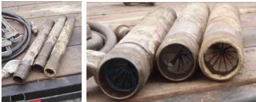
Figure 6: Split spoon heads used to create the borehole for the MDD
