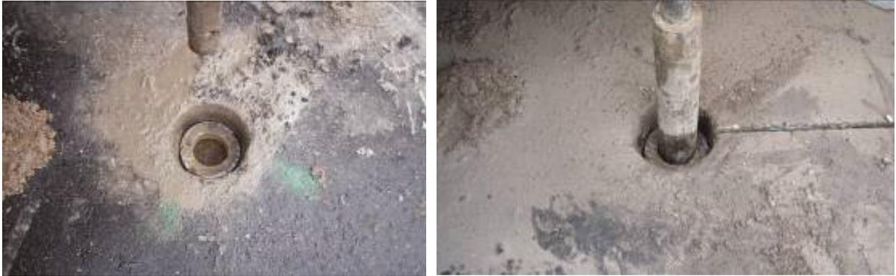
Figure 8: Wooden doughnut being used to guide the split spoon through the center of the corehole
