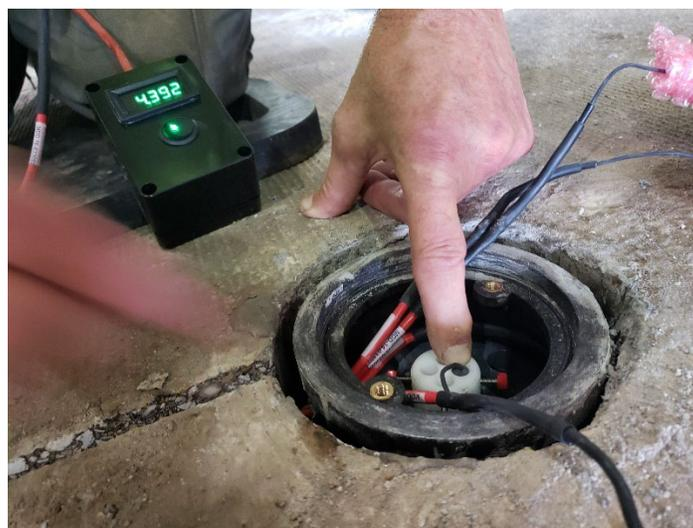
Figure 16: Sensor being installed into the sensor cavity, using the readout box to ensure that it is installed in a very slightly compressed position
