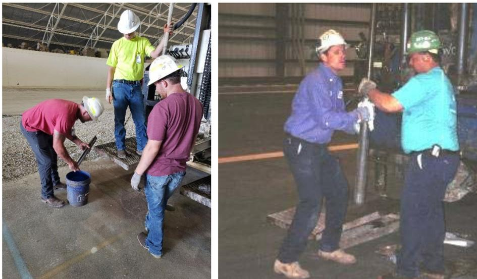
Figure 7: Left- operators cleaning the dirt from the split spoon, Right- operators putting the split spoon back onto the rig in preparation for another plunge
