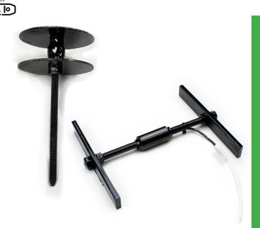
ASPHALT STRAIN TRANSDUCERS (AST/VAST) MEASURE AXIAL STRAIN IN FLEXIBLE PAVEMENT UNDER HIGH-FREQUENCY (DYNAMIC) CONDITIONS. THESE LOW-MODULUS, RUGGEDIZED SENSORS ARE BUILT TO WITHSTAND HIGH TEMPERATURES. THE **GAGE AREA HAS ARMORED PROTECTIONS FROM** VIBRATORY ROLLED COMPACTION REQUIRED FOR ASPHALT PLACEMENT.
