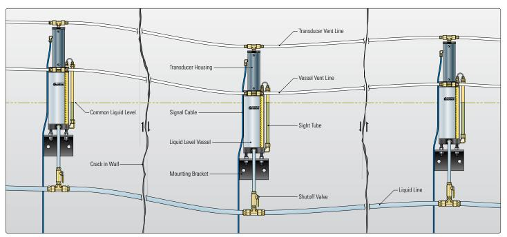
• Installation of the Model 4675 on a concrete wall with exaggerated settlement to illustrate change in elevation.
