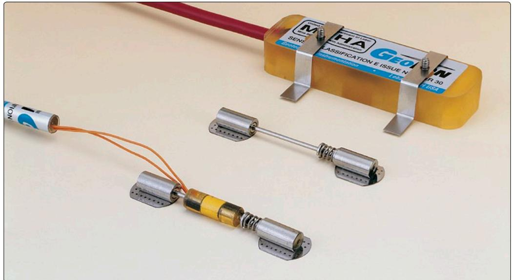
● Model 4150 (front) and Model 4100 Spot-Weldable Strain Gages.
