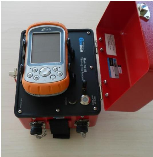
Figure12 GK405 Readout Unit
