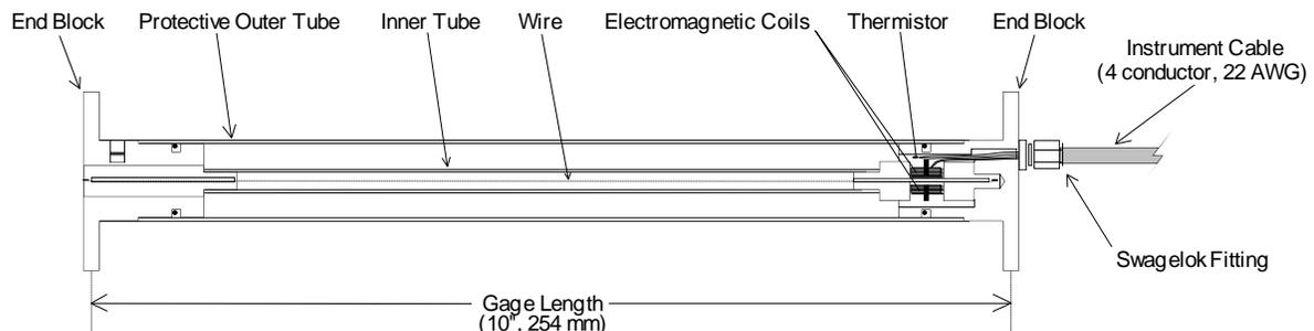
Figure 3 - Model 4210 Vibrating Wire Strain Gage
