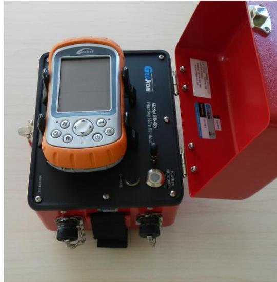
Figure 6 GK405 Readout Unit
