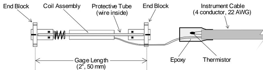
Figure 2 - Model 4202 Vibrating Wire Strain Gage
