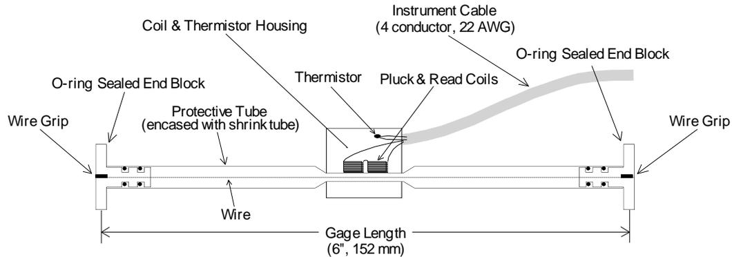
Figure 1 - Model 4200 and 4200L Vibrating Wire Strain Gage
