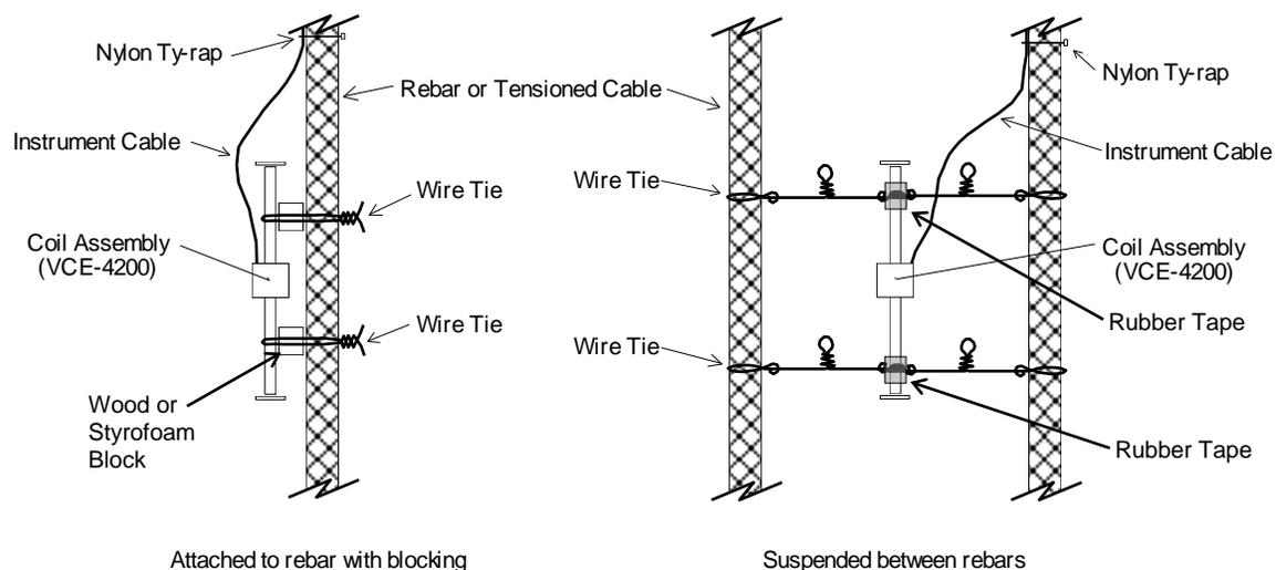
**Figure 4 - Attaching Model 4200/4200L/4200HT Strain Gages to Rebar**
