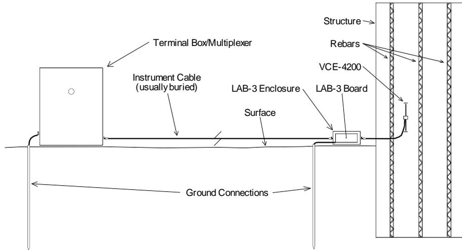
Figure 5 - Lightning Protection Scheme
