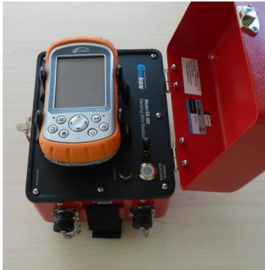
Figure 6 GK405 Readout Unit
