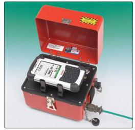
Model GK-405 Vibrating Wire Readout.
