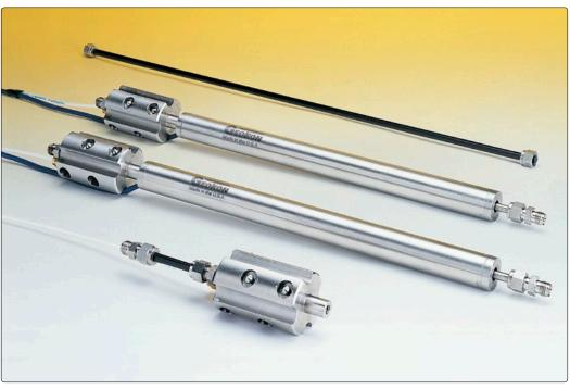
Model A-9 Retrievable Extensometer bottom anchor (front), transducer with anchor (middle two), and connecting rod (rear).
