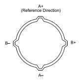
Figure 3 Inclinometer Casing
