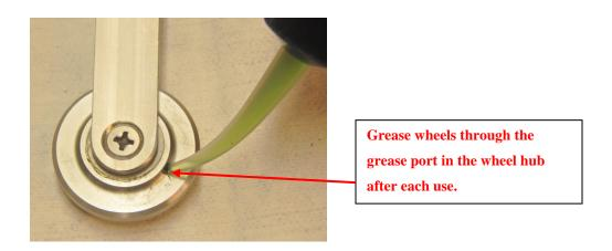
Figure 4. Wheel Lubrication
