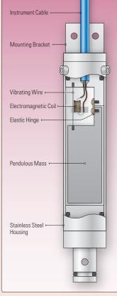
• Vibrating wire tilt sensor construction.
