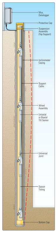
• Typical application to monitor the stability of a foundation wall.
