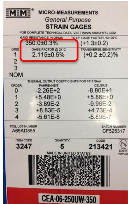
Figure 5-3 Typical micro-measurements foil gage calibration document
