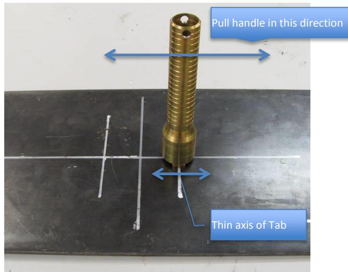
Figure 6-8 Removing a Tab with the TRT
