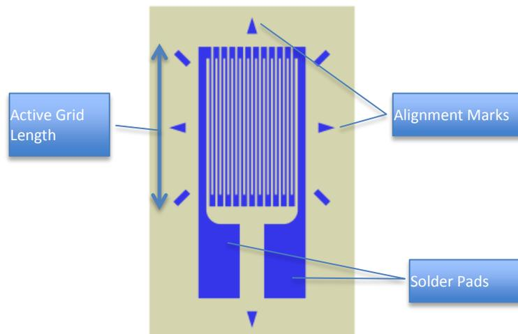
Figure 5-4 Standard Foil Strain Gage
