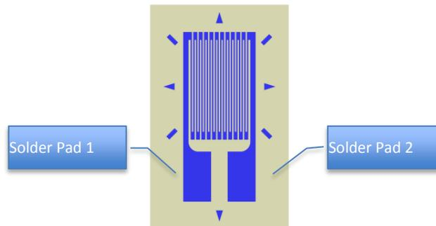
Figure 5-2 Typical 1/4-Arm foil gage
