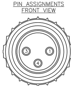
Figure 5-1 M8 connector pin assignment for three-wire connector
