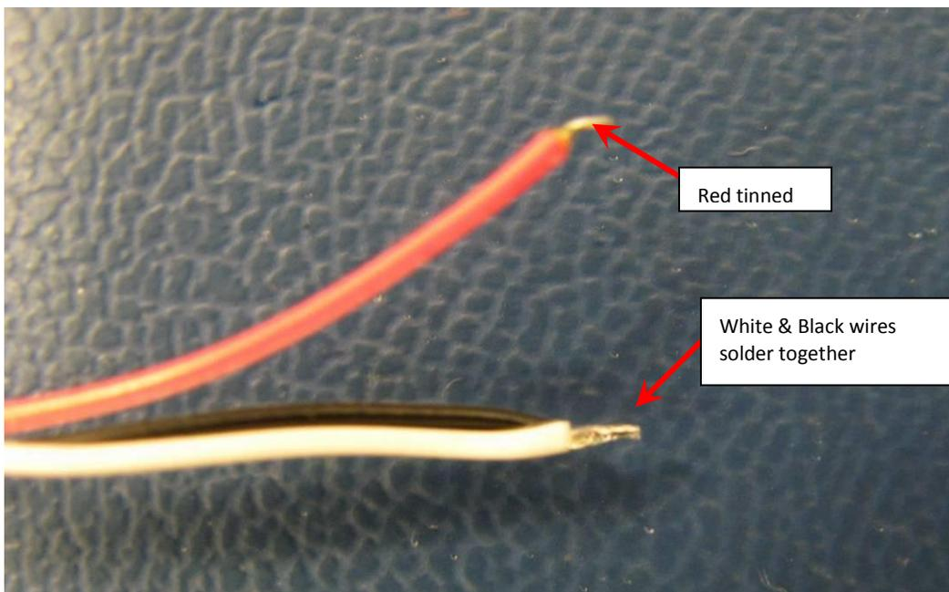
Figure 6-1Foil gage soldered lead wires.
