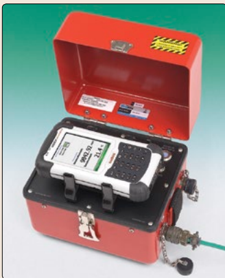
● Model GK-405 Vibrating Wire Readout for use with the Model 4900 Load Cells.
