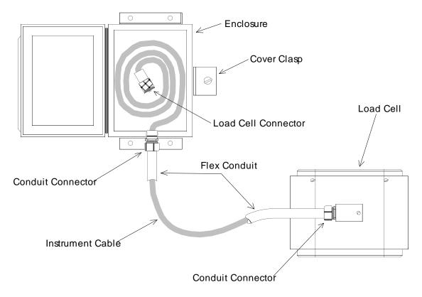
Figure 4 - Typical Load Cell System
