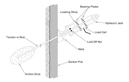
Figure 2 - Load Cells On Tiebacks For Proof Testing Only
