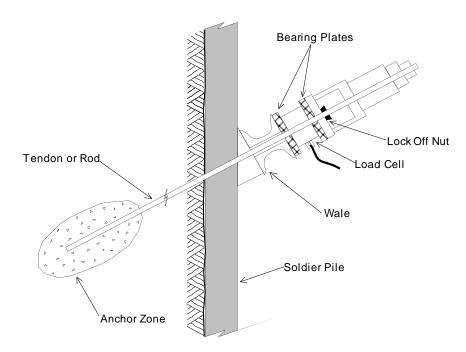
Figure 1 - Load Cells on Tiebacks for the Permanent Monitoring of Loads
