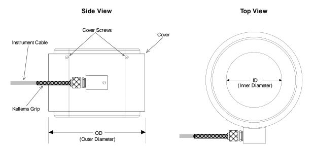
Figure 3 - Model 3000 Load Cell
