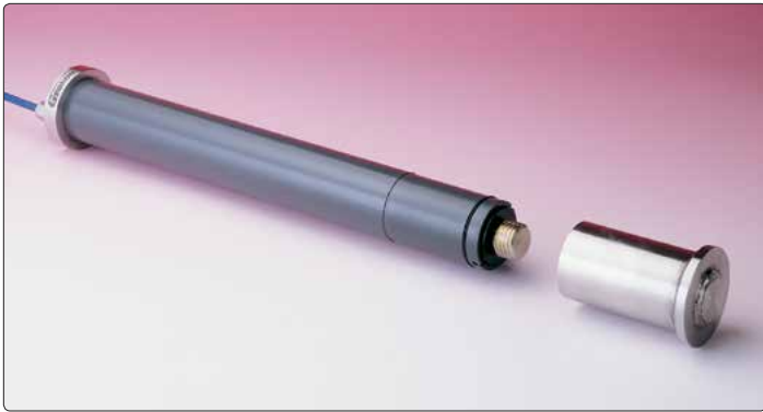
● Model 4400 Embedment Jointmeter shown with socket removed.
