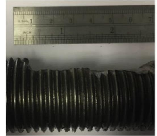
Imitation crack, by notching
