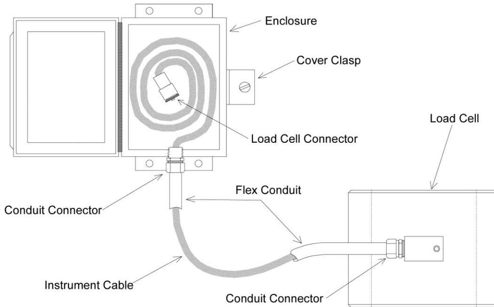
**Figure 5 - Typical Load Cell System**
