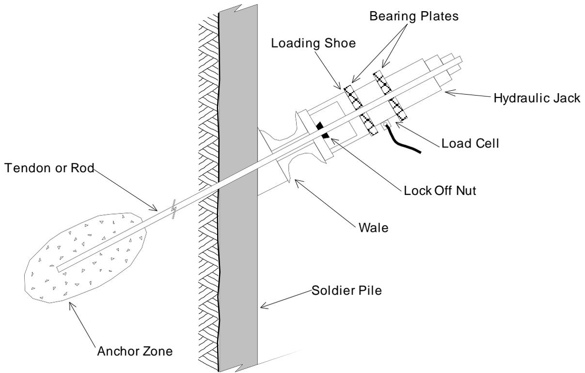
Figure 2 - Load Cell on Tieback for Proof Testing Only
