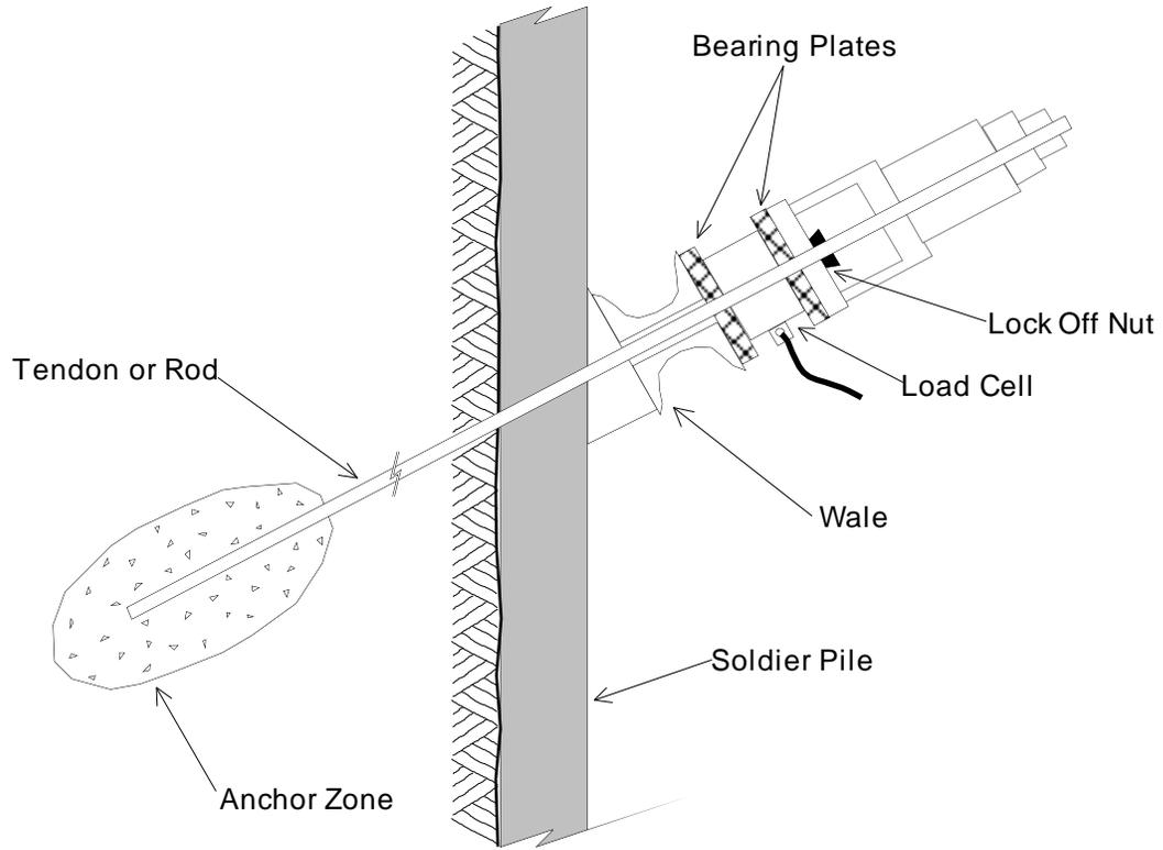
Figure 1 - Load Cell on Tieback for the Permanent Monitoring of Load
