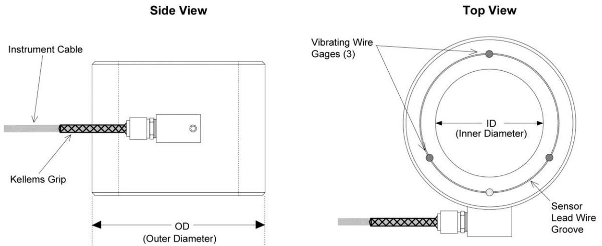
**Figure 4 - Model 4900 (3 Gage) Vibrating Wire Load Cell**
