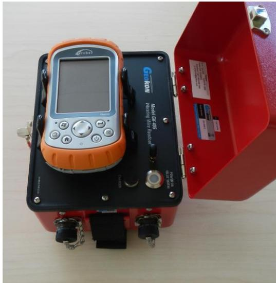
Figure 7 GK405 Readout Unit
