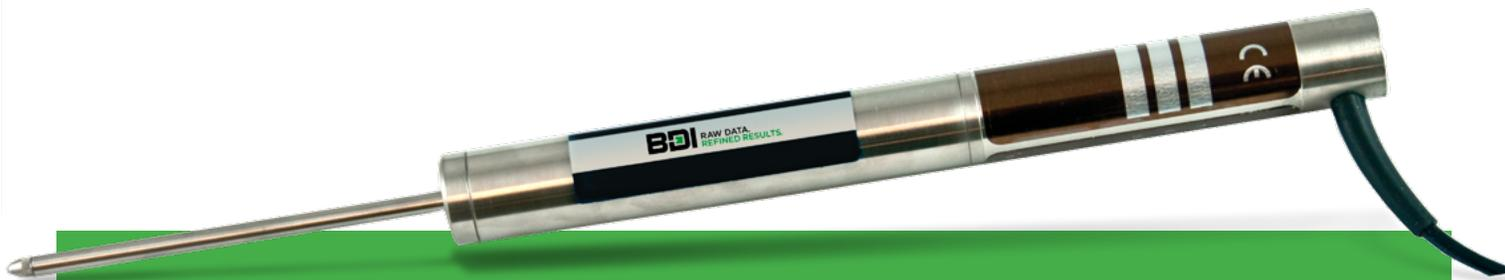
THE LINEAR VARIABLE DIFFERENTIAL TRANSFORMER (LVDT) DISPLACEMENT TRANSDUCER ACCURATELY MEASURES THE MOVEMENT BETWEEN THE SPRING-LOADED SLIDING ARMATURE AND THE EXTERIOR BODY. THESE RUGGED AND SELF-CONTAINED UNITS ARE IDEAL FOR RECORDING DISPLACEMENTS ON STRUCTURAL MEMBERS DUE TO LIVE LOADS AND TEMPERATURE VARIATIONS. WITH YEARS OF EXPERIENCE USING THESE TRANSDUCERS ON BRIDGES, BUILDINGS, AND HYDRAULIC STRUCTURES, THEY ARE THE GOLD STANDARD WHEN IT COMES TO VERY ACCURATE POSITION MEASUREMENTS.
