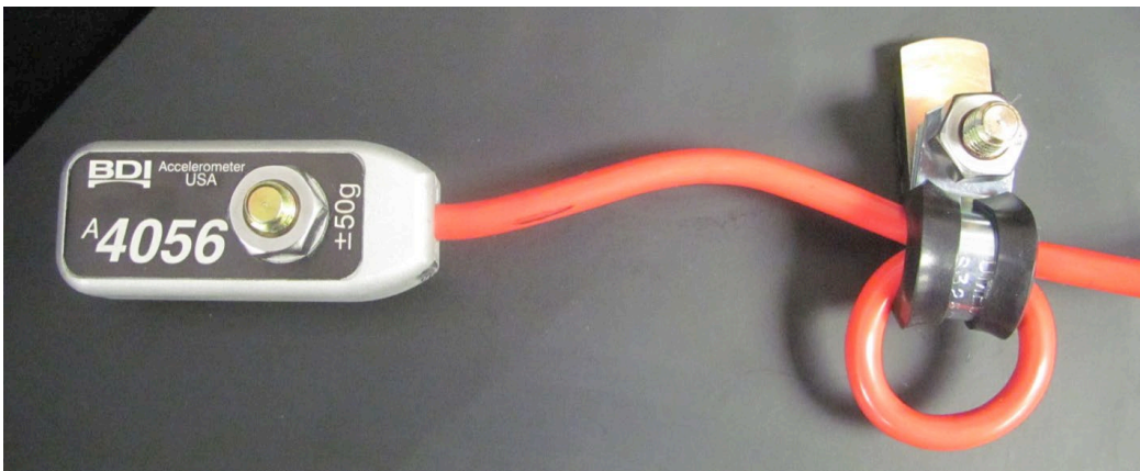
Figure 11: Sensor mounted with cable strain relief loop
