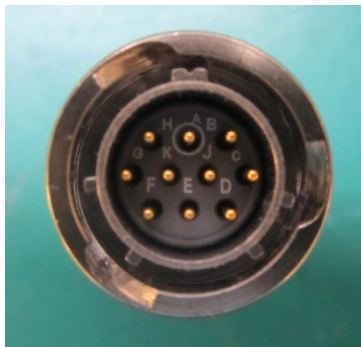
Figure 24: Intelliducer Plug Pin Assignment
