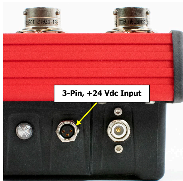
Figure 8: +24 V dc Power Input Receptacle
