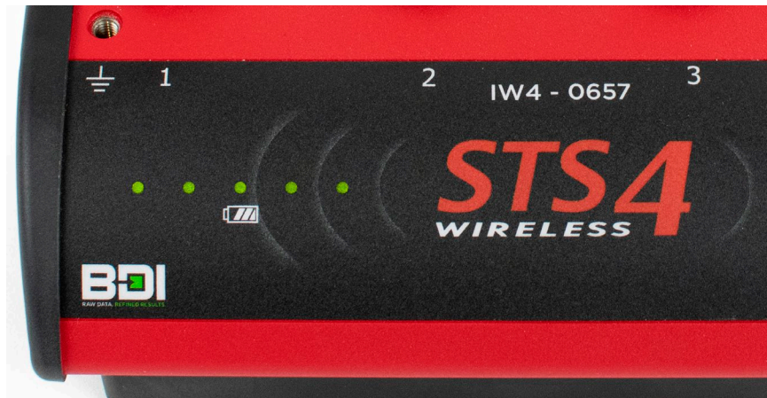
Figure 5: Battery Status LEDs
