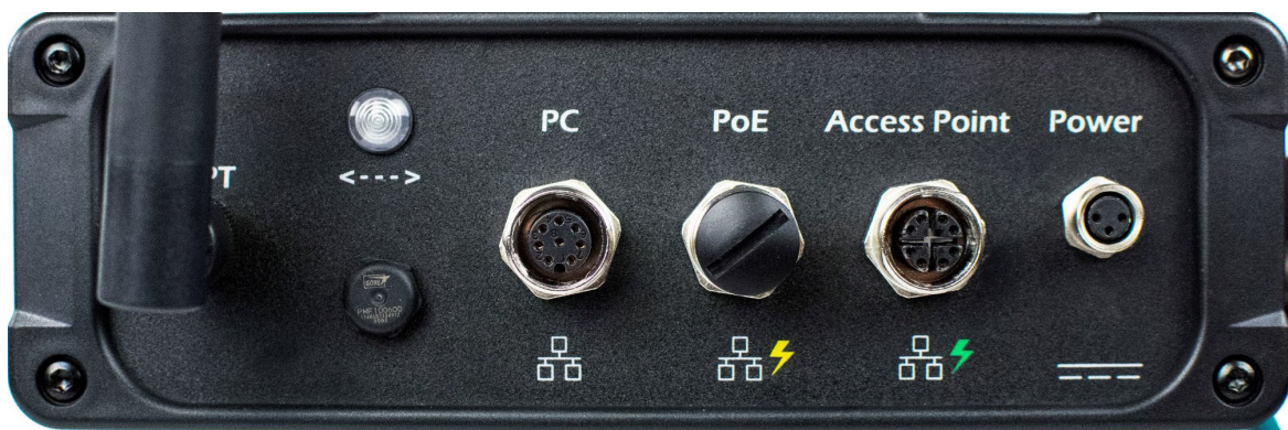
Figure 19: LAN Port Connections
