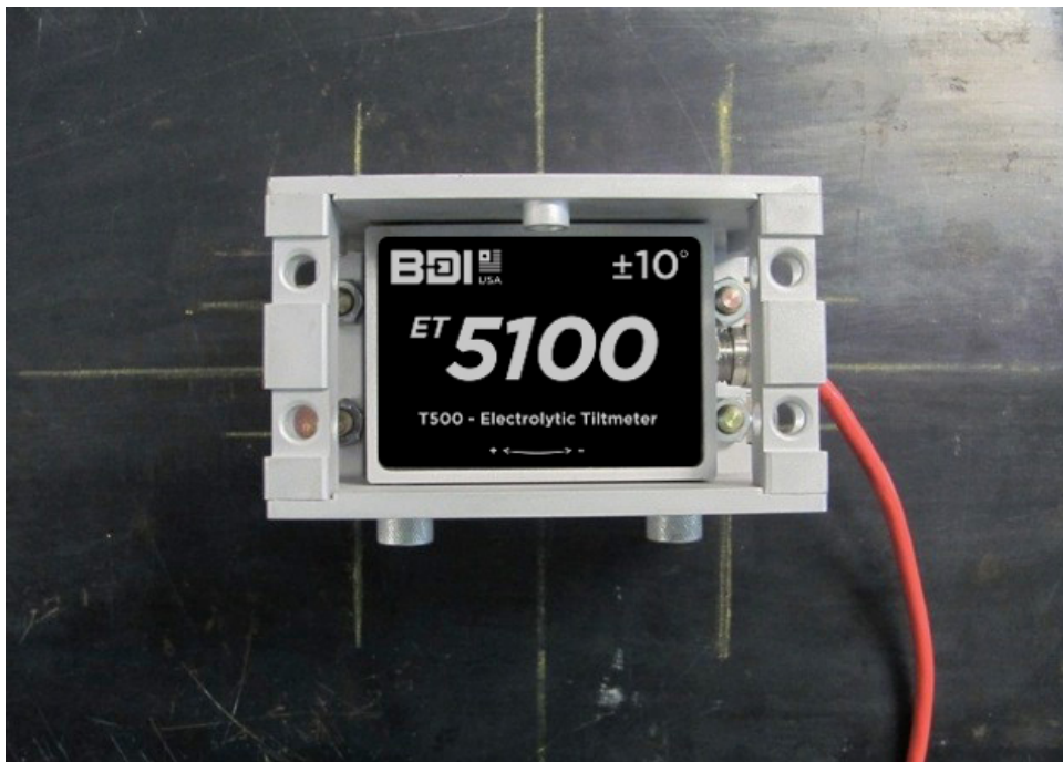
Figure 13: Tiltmeter Installed on Structural Member
