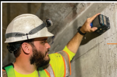
GPR for PT duct location and depth
