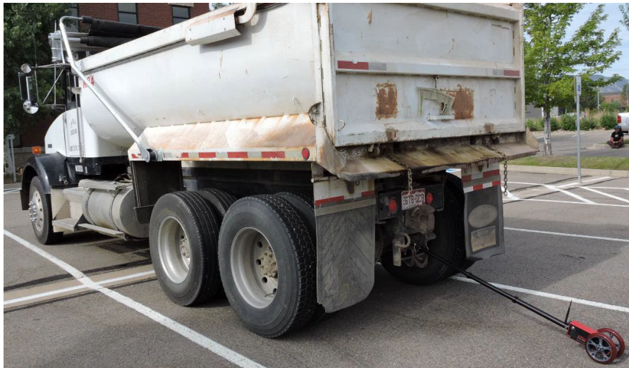
Figure 7: Typical ALPT Installation
